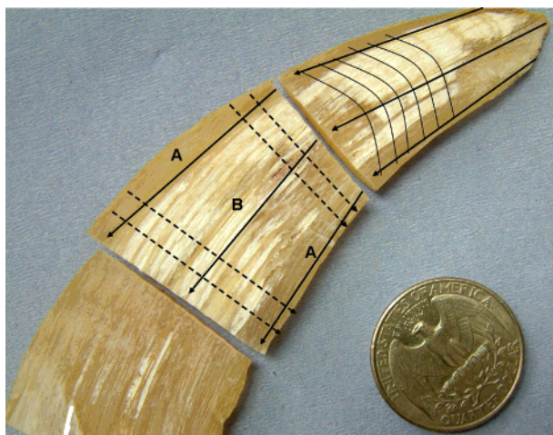
FIGURE 1. Inner surface of one of the North Ronaldsay Sheep's horn, used for laser ablation. Two different materials appear, in the cortex (A) and in the center (B) of the horn. The solid arrows indicate the scanned lines along the growth axis, while the dotted lines are the scanned cross sections.
